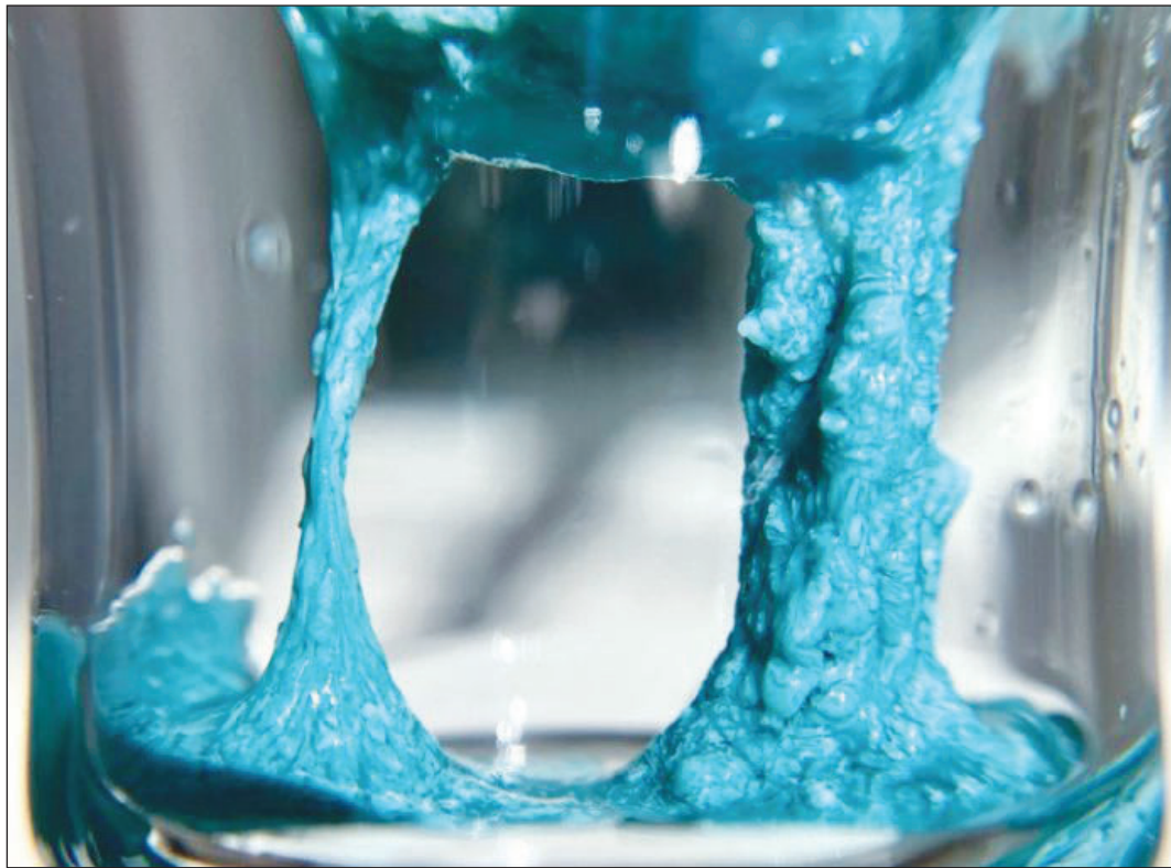
The goo developed by a trio of Northland College students could help capture metal-ion pollution from used electronics or industrial waste. It is normally colorless, but after binding to copper ions the goo turns bright turquoise. (Contributed photo)
