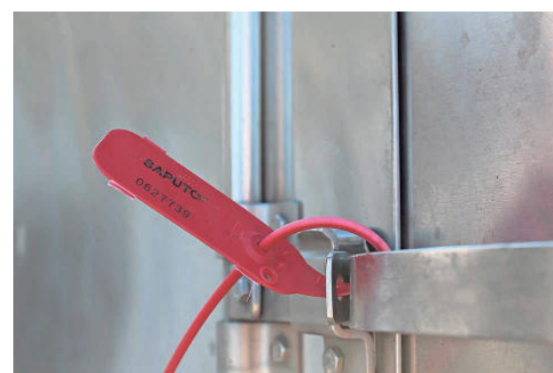
A seal is placed on the rear of the milk tanker to ensure that the milk inside has not been tampered with. COLLEEN KOTTKE / WISCONSIN STATE FARMER
