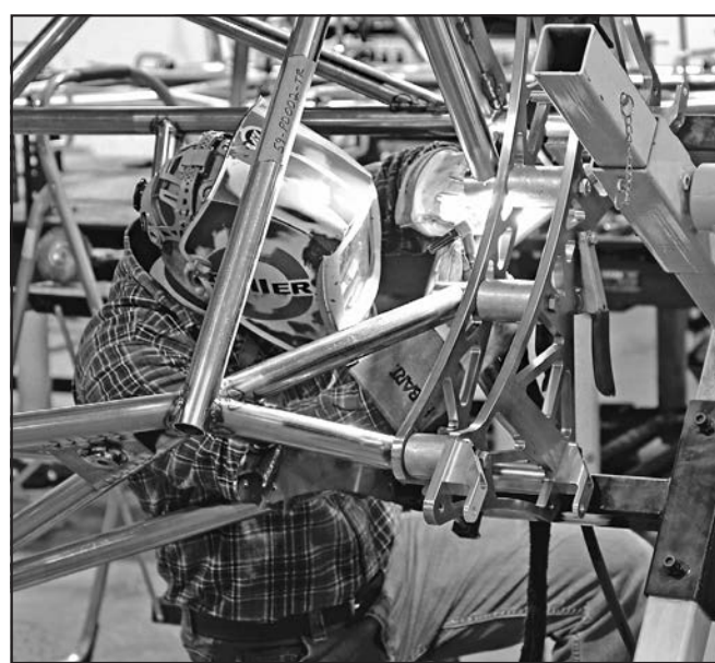
The Indy Special's custom spaceframe chassis is welded together at the manufacturing facility in Three Lakes.
