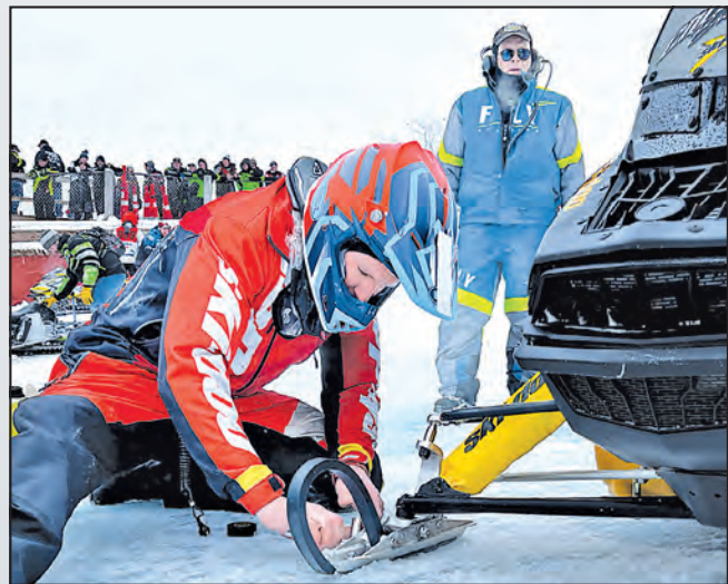
Matt Goede works quickly to change his front right carbide during a red flag Sunday. —Staff Photo By DOUG ETTEN
