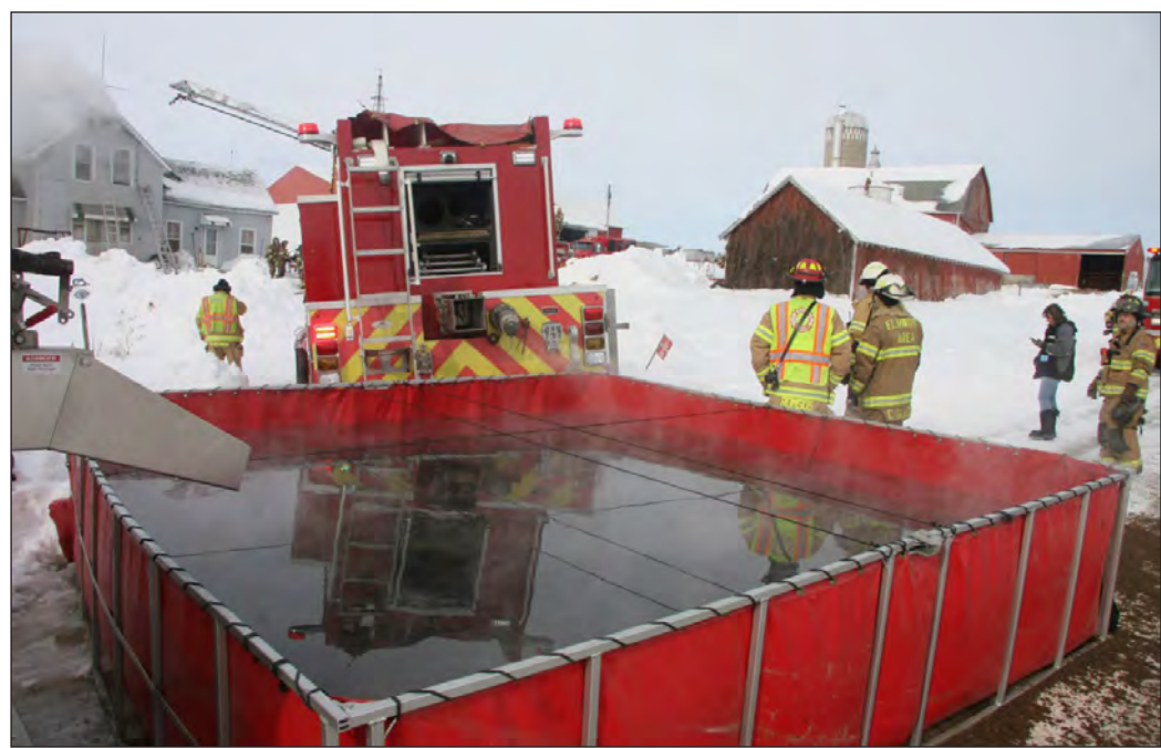
One of two drop tanks providing water at the scene of a house fire Saturday, Jan. 28 on 320 th Avenue in the town of Cady, east of Spring Valley. Submitted photo
