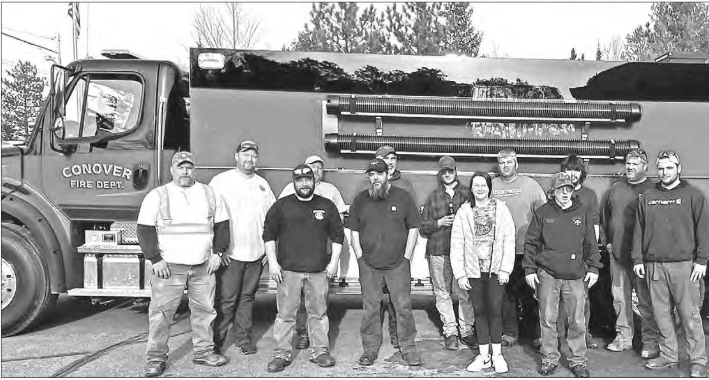
The Conover Fire and Rescue Departments recently received an All-Poly Series Tanker-Pumper to add to the organization's equipment. The apparatus features a Freightliner M2-112 Chassis, a Hale AP50 PTO Side Kick Pump and a 4000 Gallon APR Fire Tank purchased from Midwest Fire out of Luverne, Minn. During
