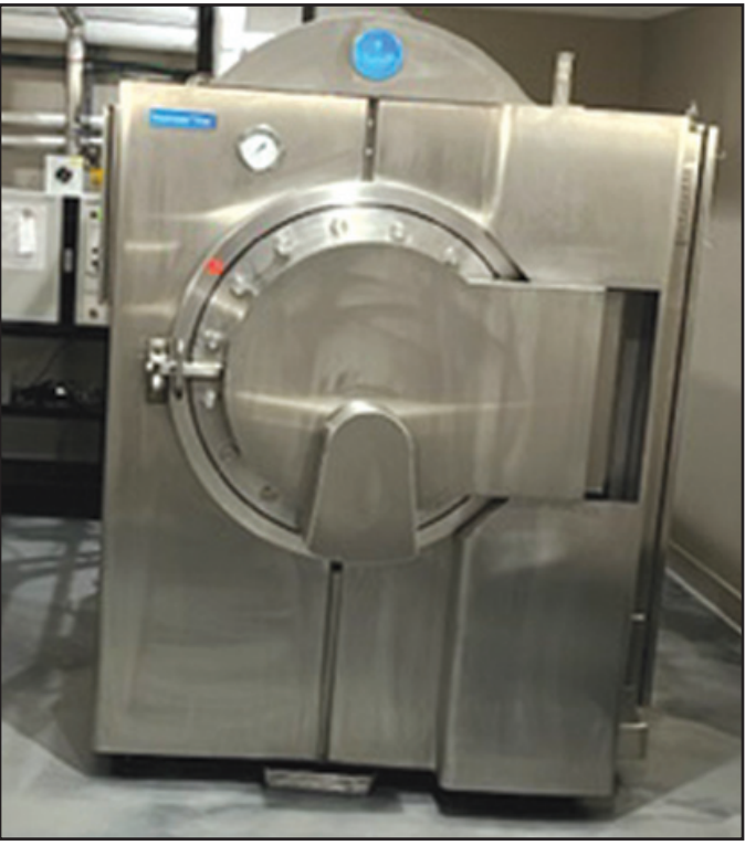
After the water cremation process, bones left over which can either be given to the family, or crushed into an ash like powder for the burial ceremony. Below is the tank used for water cremation that is filled with water and 5% potassium hydroxide where the body is placed for and the tissues are softly dissolved.
