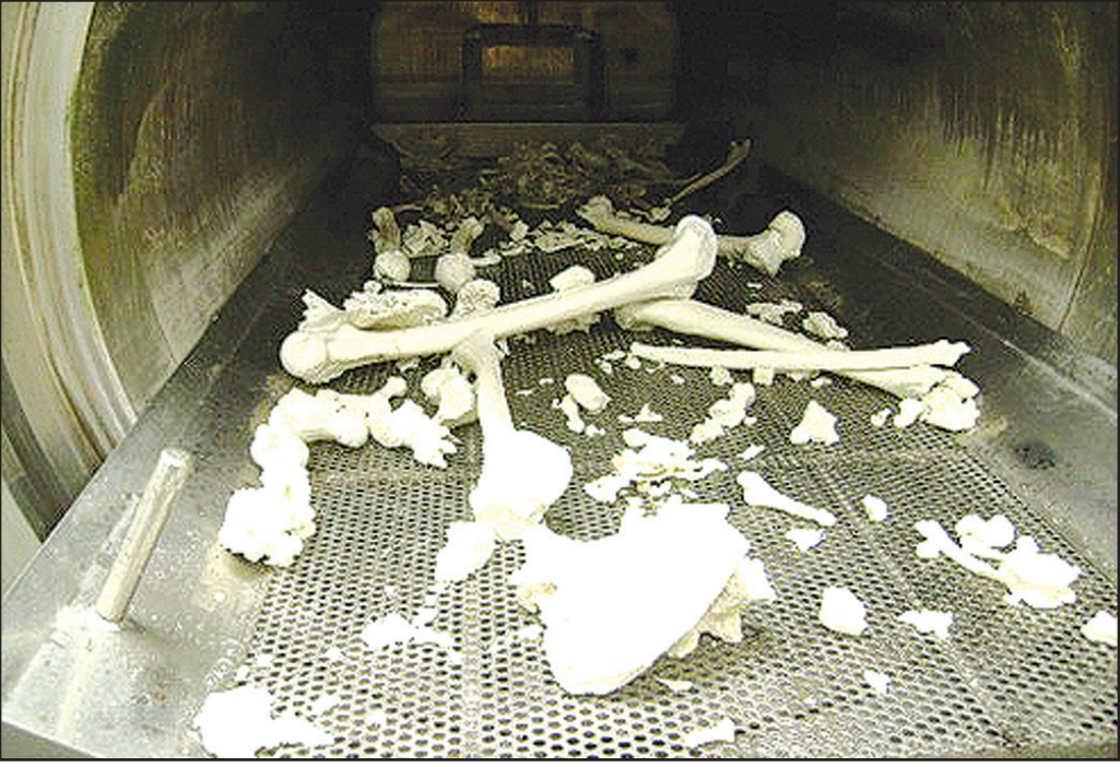
After the water cremation process, bones left over which can either be given to the family, or crushed into an ash like powder for the burial ceremony. Below is the tank used for water cremation that is filled with water and 5% potassium hydroxide where the body is placed for and the tissues are softly dissolved.
