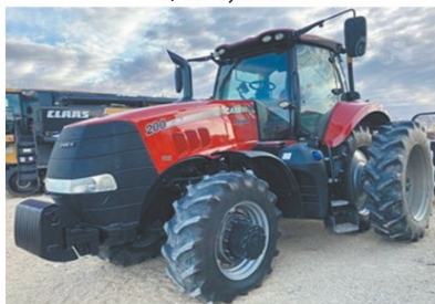
2015 CASE IH MAGNUM 200 2200 hours, 18.4-46 Duals, 19 Speed PS, Susp. Front Axle, 3Pt, 540/1000 PTO, 4 Valves, Luxury Cab, Guidance Rdy $137,500 + 0% for 12 months
