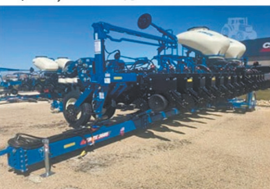
2022 KINZE 3605 16/31 Twin-Line, Bulk-Fill, 31 No-Till Coulters & Soybean Meters, KPM III Monitor, Markers, Mechanical Drive $184,500 + LOW RATE FINANCING
