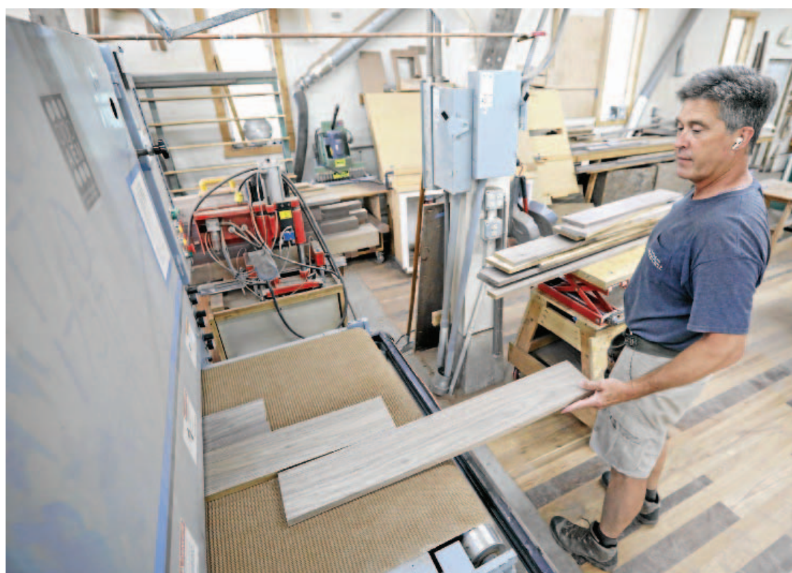
Andy Lynch puts pieces of walnut to be used for a cabinet into a sanding machine at The Wood Cycle of Wisconsin in Oregon.
